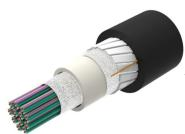
Fiber indoor/outdoor cable, All-Dielectric, LSZH Riser-Rated, 144 fiber, Gel-Free, Central Tube Rollable Ribbon, Singlemode G.657.A2/B2, Feet jacket marking, Black jacket color, Cca flame rating
