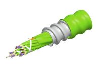
Fiber indoor cable, LazrSPEED® Riser/LSZH rated MPO Trunk, interlocking aluminum armored, 72 fiber multi-unit with 12 fiber subunits, Feet jacket marking, Lime-green jacket color
