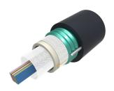
Fiber OSP cable, Steel Armored, Arid-Core, Dry Central Tube Ribbon, 12 fiber, Multimode OM3, bend insensitive, Feet jacket marking, Black jacket colorv
