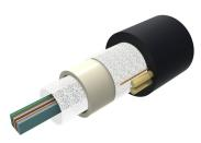
Fiber OSP Cable, Non-Armored, All-Dielectric, Arid-Core, Dry Central Tube Ribbon, 36 fibers, Singlemode G.652.D and G.657.Al, Gel-free, Feet jacket marking, Black jacket color
