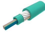
Fiber Indoor Cable, LSZH Riser, All-Dielectric, Central Tube Ribbon, Multimode, OM4, bend insensitive, 12 Fibers, Gel-free, Feet jacket marking, Aqua jacket color
