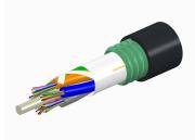
Fiber OSP cable, TeraSPEED® Single Jacket/Single Armor, Gel-Free, Stranded Loose Tube, 72 fibers, Composite OM3 and G.652.D and G.657. A1, Feet jacket marking, Black jacket color
