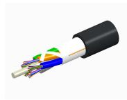
Fiber OSP cable, TeraSPEED® Single Jacket All-Dielectric, 84 fiber, Gel-Free, Outdoor Stranded Loose Tube w/HDPE Outer Jacket, Singlemode G.652.D and G.657.Al, Feet jacket marking, Black jacket color
