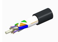
Fiber OSP cable, TeraSPEED® Single Jacket All-Dielectric, 72 fiber, Gel-Free, Outdoor Stranded Loose Tube w/HDPE Outer Jacket, Singlemode G.652.D and G.657.A1, Feet jacket marking, Black jacket color
