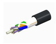
Fiber OSP cable, TeraSPEED® Single Jacket All-Dielectric, 48 fiber, Gel-Free, Outdoor Stranded Loose Tube w/HDPE Outer Jacket, Singlemode G.652.D and G.657.Al, Feet jacket marking, Black jacket color
