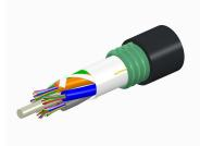
Fiber OSP cable, TeraSPEED® Single Jacket/Single Armor, 168 fiber, Gel-Free, Stranded Loose Tube, Singlemode G.652.D and G.657.A1, Feet jacket marking, Black jacket color
