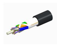
Fiber OSP cable, TeraSPEED® Single Jacket All-Dielectric, Gel-Free, Stranded Loose Tube, 72 fibers, Composite OM3 and G.652.D and G.657. Al, Feet jacket marking, Black jacket color
