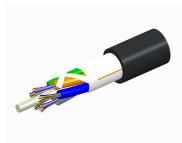
Fiber OSP cable, TeraSPEED® Single Jacket All-Dielectric, Gel-Free, 4 fiber, Stranded Loose Tube, Singlemode G.652.D and G.657.Al, Feet jacket marking, Black jacket color
