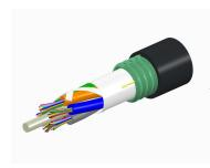
Fiber OSP cable, TeraSPEED® Single Jacket/Single Armor, 288 fiber, Gel-Free, Stranded Loose Tube, Singlemode G.652.D and G.657.Al, Meters jacket marking, Black jacket color
