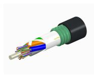
Fiber OSP cable, TeraSPEED® Single Jacket/Single Armor, 156 fiber, Gel-Free, Stranded Loose Tube, Singlemode G.652.D and G.657.A1, Feet jacket marking, Black jacket color
