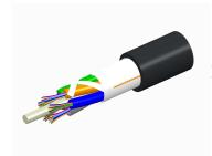
Fiber OSP cable, LazrSPEED® Single Jacket All-Dielectric, Gel-Free, Stranded Loose Tube, 24 fibers, Multimode OM4, Feet jacket marking, Black jacket color
