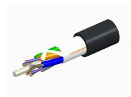
Fiber OSP cable, LazrSPEED® Single Jacket All-Dielectric, Gel-Free, Stranded Loose Tube, 24 fibers, Multimode OM3, Feet jacket marking, Black jacket color
