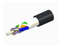
Fiber indoor/outdoor cable, TeraSPEED®, Single Jacket All-Dielectric, Low Smoke Zero Halogen (LSZH), 48 fiber, Multimode/Singlemode, Gel-Free, Stranded Loose Tube, Black jacket color, Feet cable marking, Eca flame rating
