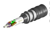
Fiber indoor/outdoor cable, LazrSPEED®, Plenum Rated, Gel-Free, Stranded Loose Tube with Aluminum Interlocking Armor containing a Plenum Rated Outer Jacket, 144 fiber, Multimode OM4, Feet jacket marking, Black jacket color
