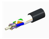
Fiber indoor/outdoor cable, TeraSPEED®, Single Jacket All-Dielectric, Low Smoke Zero Halogen (LSZH), 96 fiber, Singlemode G.652.D and G. 657.A1, Gel-Free, Stranded Loose Tube, Black jacket color, Feet cable marking, Eca flame rating
