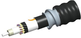
Fiber indoor/outdoor cable, LazrSPEED® Low Smoke Zero Halogen Riser MPO Trunk, interlocking aluminum armored, Multimode OM4, 72 fiber multi-unit with 12 fiber subunits, Gel-free, Feet jacket marking, Black jacket color
