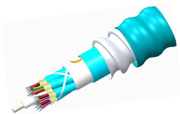
Fiber indoor cable, TeraSPEED® Riser Distribution, interlocking aluminum armored, Multimode/Singlemode, 48 fiber multi-unit with 12 fiber subunits, gel-free, Feet jacket marking, Aqua jacket color
