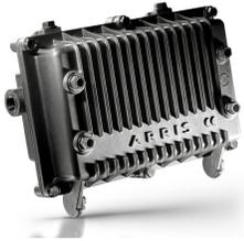
STARLINE® BLE120 Broadband Line Extender, 1.2 GHz GaN output w /38 dB gain, 5-204 MHz/258-1218 MHz Bandpass split, 27 dB Upstream gain, Standard housing (full station), Powering option X
