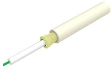
Indoor/Outdoor Fiber Optic Drop cable, 1 Fiber G657.B3 0.9mm tight buffer. Breaking load Max 2000N. Suitable for installation under overhead power lines  $\leq 11\text{kV}$ , vertical clearance  $\geq 1.8\text{m}$ .
