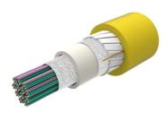
Fiber indoor cable, All-Dielectric, Riser-Rated, Gel-Free, Central Tube with 12x200um Rollable Ribbons, 1728 fiber, G.652.D / G.657.A1 Singlemode, Feet jacket marking, Yellow jacket color
