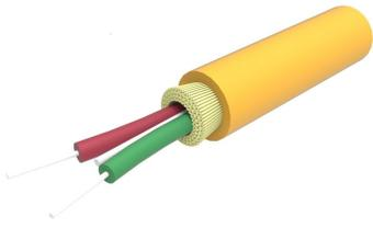
Fiber Indoor/Outdoor Drop Cable, FTTH, 2 fibers, Singlemode, G.657.A2, Gel-free, Meters jacket marking, Yellow jacket color, Dca Flame Rating
