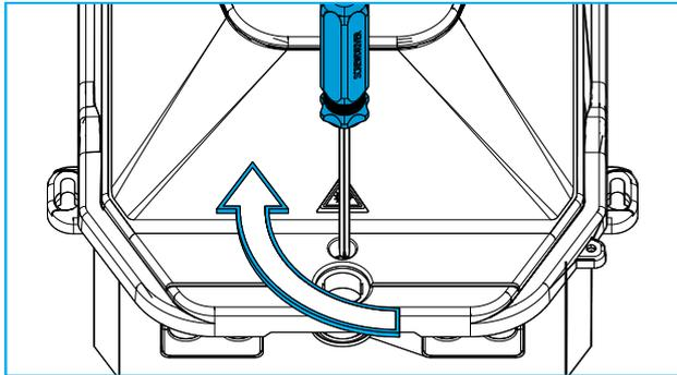
1 Secure by turning the locking screw.
