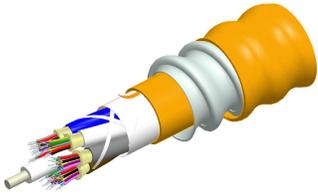
Fiber indoor cable, OptiSPEED® Plenum Distribution, interlocking aluminum armored with plenum jacket, 6 fiber single-unit, Gel-free, Multimode OM1, Feet jacket marking, Orange jacket color
