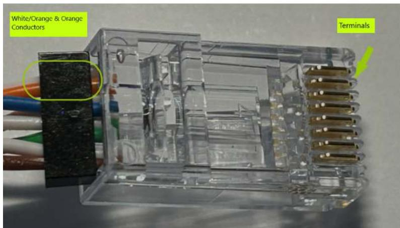
2.4 Fully insert prepared cable and load bar into the plug:
