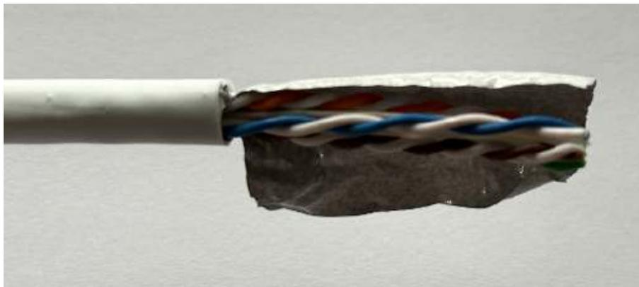
1.4 Separate the twisted pairs and center core:
