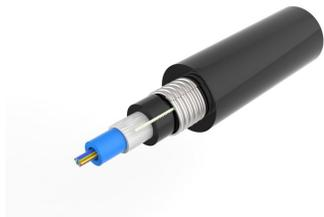
Fiber Indoor/Outdoor cable, TeraSPEED®, 120 min Fire Survival, Low Smoke Zero Halogen (LSZH), 24 fiber, Gel-Filled, Central Loose Tube, Singlemode G.652.D and G.657.A1, Meters jacket marking, Black jacket color. Provides Rodent Resistance.
