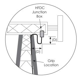
**Reminder:** Plan grip location by measuring distance (D) from Fiber Enclosure Box to tower support member.
