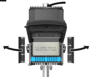
Release the lower latches using a flat faced screwdriver on the sides of the junction box and lift the bottom half to open. Carefully clip open the front panel by engaging the clip located at the top. This will provide easy access to the internal components. Remove packaging foam from inside the junction box and ensure all connections are intact.
