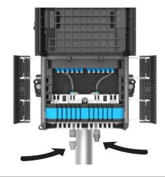
Gently remove the dust caps from the HFMOC connectors located at the bottom of the junction box. Ensure that the connectors remain clean and free from contaminants during the process. Carefully remove the dust caps from the HFMOC connectors on the FT-24CGAHBN series cable, taking care not to touch or contaminate the fiber ends.
