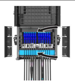
Connect the outgoing fiber jumper DLC (Gen 1.5 push pull) connectors into the adapter plate. Route the cables through the appropriate gel gland points of the junction box. Ensure proper strain relief to avoid damage to the cables. Be careful to maintain the correct bend radius for the fiber cables to prevent signal loss or damage.
