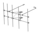
G22HDX Tower Sector Frame with extended face, 15 ft x 2.88 in OD face pipes. Base Kit Only. Includes five 2.88 OD x 120 in antenna pipes
