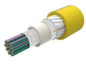
Fiber indoor cable, All-Dielectric, LSZH/Riser-Rated, Gel-Free, Central Tube 200µm Rollable Ribbon, 864 fiber, Singlemode G.657.A2/B2, Feet jacket marking, Yellow jacket color, Cca flame rating
