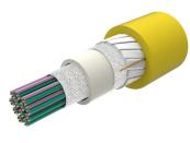
Fiber indoor cable, All-Dielectric, LSZH/Riser-Rated, Gel-Free, Central Tube 200µm Rollable Ribbon, 288 fiber, Singlemode G.657.A2/B2, Feet jacket marking, Yellow jacket color, Cca flame rating
