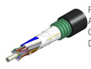
Fiber indoor/outdoor cable, TeraSPEED® Mini Single Jacket/Single Armor, Riser/LSZH rated, 144 fiber, Singlemode G.652.D and G.657.A1, Gel-Filled, Stranded Loose Tube, Black jacket color, Feet jacket marking, Dca flame rating
