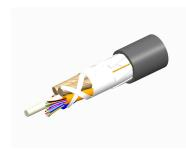
Fiber indoor/outdoor cable, LazrSPEED®, Single Jacket All-Dielectric, Plenum Rated, Gel-Free, Stranded Loose Tube, 36 fiber, PVDF jacket, Multimode OM3, Black jacket color, Feet cable marking
