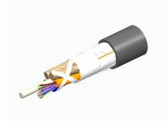
Fiber indoor/outdoor cable, LazrSPEED®, Single Jacket All-Dielectric, Plenum Rated, , 12 fiberMultimode OM4, Gel-Free, Stranded Loose Tube, PVDF jacket, Black jacket color, Feet cable marking
