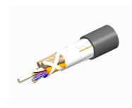
Fiber indoor/outdoor cable, LazrSPEED®, Single Jacket All-Dielectric, Plenum Rated, Multimode OM4, Gel-Free, Stranded Loose Tube, PVDF jacket, 96 fiber, Black jacket color, Feet cable marking
