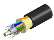
Fiber Indoor/Outdoor cable, Composite Plenum Distribution, 18 fiber single-unit, Composite OM4 and G.652.D and G.657.A1, Gel-free, Feet jacket marking, Black jacket color
