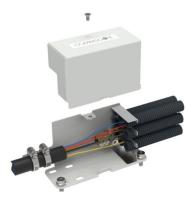
Cable unit break out kit for low to medium fiber count loose tube cables (max 24mm), 1 cable to max 6 flex tubes (ID 12mm). Cable application range subject of loose tube diameter and stiffness (indicatively: max 864f cable with 1,7mm loose tube)
