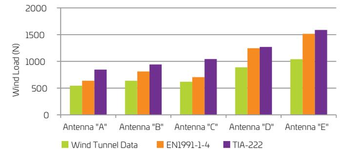
Figure 8. Maximum wind load at 150 km/h
