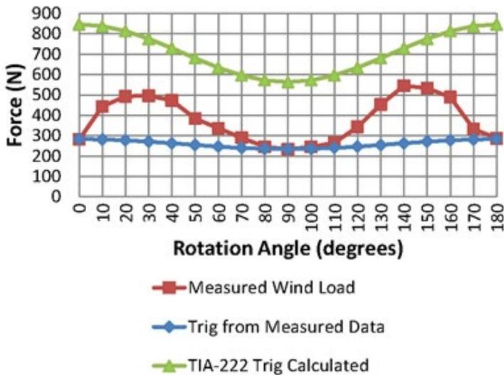
Figure 11. Three methods of calculating wind loads at angles between 0 and 180 degrees
