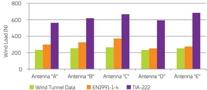
Figure 7. Lateral wind load at 150 km/h
