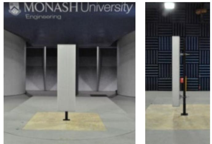
Figure 3. Antenna testing inside Monash Wind Tunnel Research Platform
