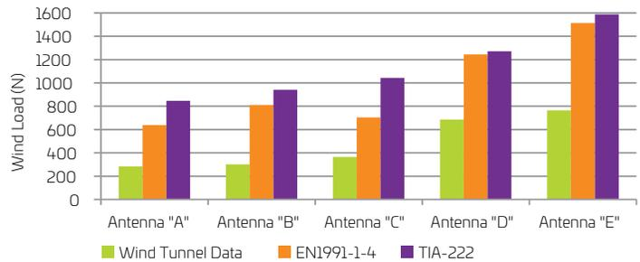
Figure 6. Frontal wind load at 150 km/h
