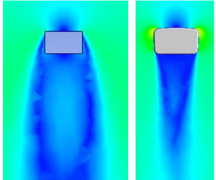
Figure 2. CFD results between basic rectangle and optimized radome
