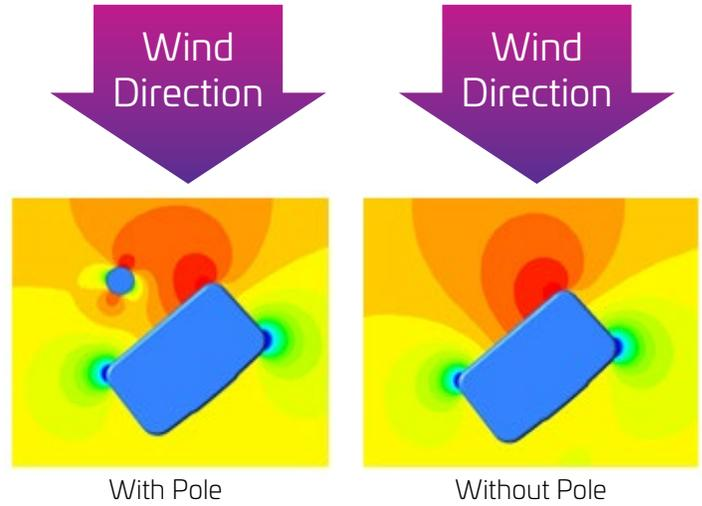
Figure 12. CFD illustrates the pole's effect on antenna wind loading
