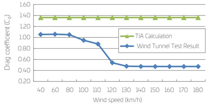
Figure 5. Drag coefficient versus velocity
