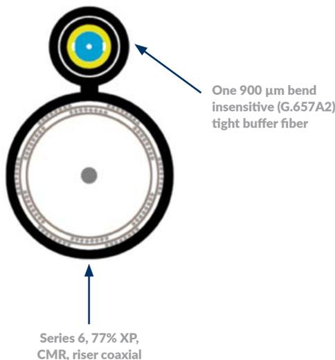
This family of electrical and optical hybrid products offers a combination of coaxial cables paired with optical fiber. The siamese configuration allows for a coaxial installation now with the capability to go to fiber at any time in the future (or, if needed, the fiber can be installed now). This is an ideal product choice that saves installation costs, ensuring future migration strategies including PON, RFoG and other FTTx technologies.
