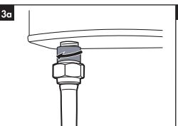
Thread HSG-M29-ADPT to the 7/16 DIN male coupling nut in counter-clockwise direction. Adapter needs only to make slight contact with 7/16 DIN Male coupling nut.
