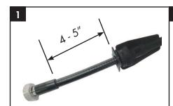
Route and form the jumper assembly with HELIAX® SureGuard weatherproofing system installed prior to attaching the coupling nuts. Make sure that the HSG boot is approximately 4 to 5 inches below the bottom of the molded portion of the jumper.
