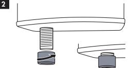
If component has a fully threaded 7-16 DIN female you must first thread HSG-M29-ADPT onto the device port in a clockwise direction (be sure not to cross thread). Adapter does not need to be threaded to the base of component, it needs to allow the DIN Male coupling nut to be torqued to specification without obstruction.
