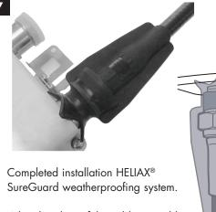
When bending of the cable assembly maintain 2 inches of straight cable length behind the connector strain relief overmold. Do not hold the connector and bend the cable directly behind it, rather hold the cable adjacent to the connector to keep stress from the cable/connector junction.
