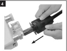
Pull the ribs outward and slide the boot over the connector.
