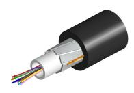
Fiber OSP cable, PE, Gel-filled Central Tube, 12 fiber, Singlemode G.657. Al, Meters jacket marking, Black jacket color
