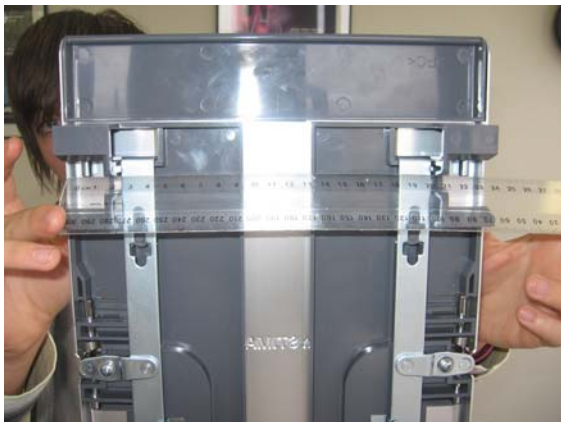
Figure 1. VTC Door Hinge Pin Spacing
