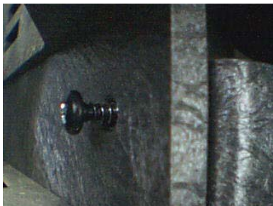
To install the packing loosen attachment screws
