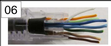
Untwist all wire pairs and Add Twist to Orange and Brown pairs to align with Step 7. Make sure No Twist in Blue and Green pairs back to jacket.
