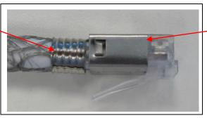
Shield end against raised edge of plug housing
