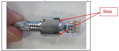
Figure 12. Orient Shield
