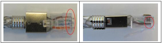
Figure 11. Verify Conductors are Fully Inserted
