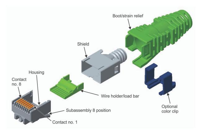
Figure 1. Slim-Line Modular Plug Components
