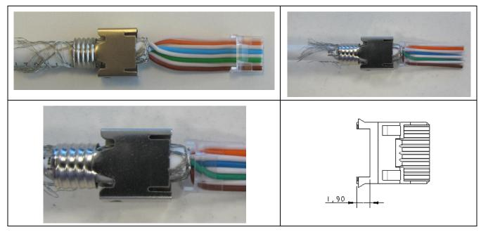
Figure 7. Insert Conductors through Wire Holder
