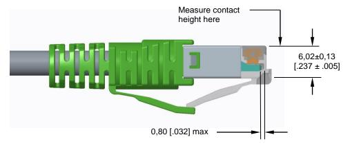
Figure 16. Plug Tolerances
