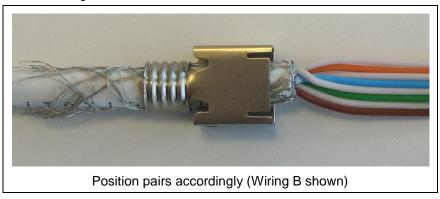
Figure 5. Cable Positioning
