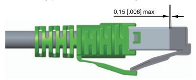
Figure 17. Gap Between Shield and Housing
