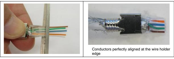
Figure 8. Trim Conductors Even with Wire Holder
