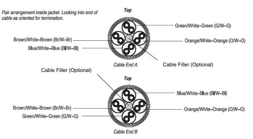
Figure 2. Arrangement of Color-Coded Pairs
