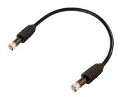
HELIAX® 1/2" SureFlex® Jumper with interface types 7-16 DIN Male and 7-16 DIN Female with HELIAX® SureGuard weatherproofing, 1.5 m (boot on DM end only, DF end no boot)
