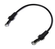
D-CLASS LDF4-50A SureFlex® Jumper with interface types 4.3-10 Male and 4.3-10 Male with HELIAX® SureGuard weatherproofing, 5 m
